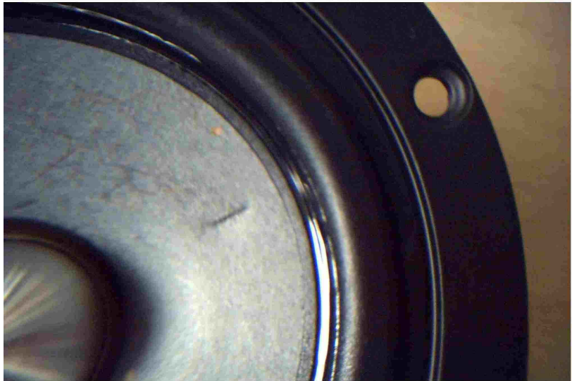
Illustration 3: One each of the two opposing pair of dimples. Longer dimple in top image, shorter dimple in the lower image. Illustration 3: One each of pair of long and short dimples embossed on diaphragm
